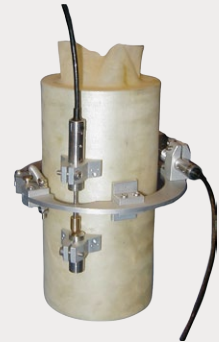
Fig. 2 LVDT transducers as shown on sample.
